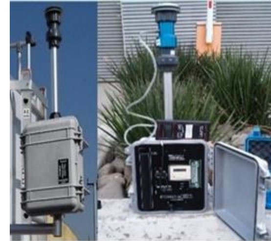
PM10 Sampling using the Minivol sampling device. Source: Own elaboration from photographs taken at the study site.
