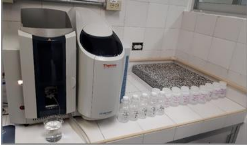
Atomic Absorption Spectrophotometer, Thermo Scientific Brand, model iCE 3000 Series AAS used in this work. Source: Own elaboration from pictures taken in the Laboratory.
