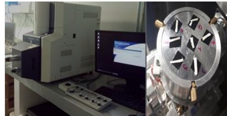
Electronic Microscope used for the elemental and morphological analysis of PM10 particles and view of the filters mounted on the equipment. Source: Own elaboration from pictures taken in the Laboratory.
